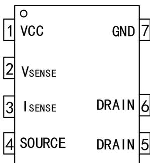
Figure2.1: G5238MK Series (7 Lead SOP7 Package)
