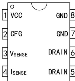
Figure2.1: G5139P Series (8 Lead DIP8 Package)
